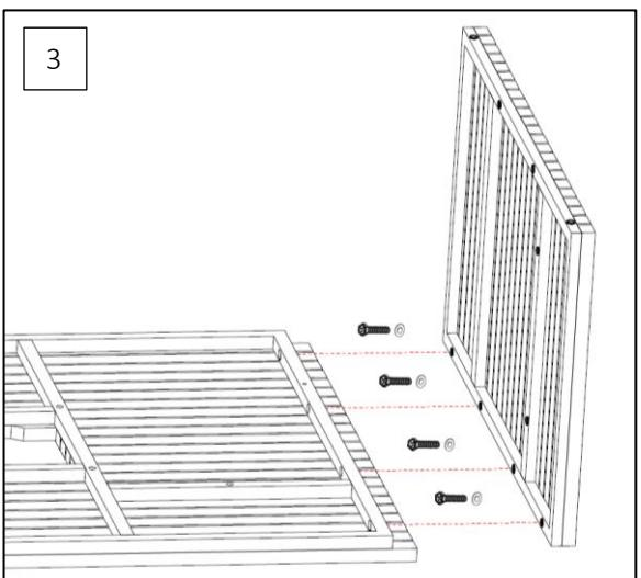
4. Then attach the second side panel C to tabletop A (see indication C) using 4x K and 4x I.
