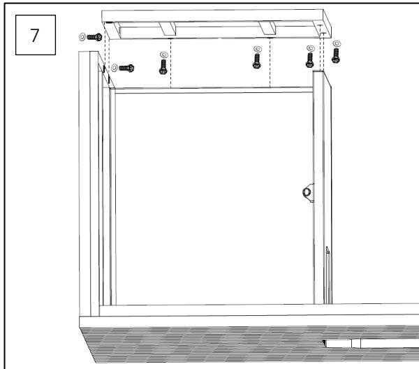
8. The support for the gas cylinder **G** can now be mounted. Position the support so that the stainless steel pin on the door **F** fits into the recess of the support **G**. Then proceed to the next step.
