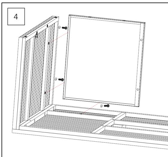
5. Please note: the table has been turned 180°. Mount the rear panel of the gas cylinder unit E to side panel C using 2x J and 2x I. Afterwards, attach rear panel E to the aluminium beam on tabletop A using 1x J and 1x I.
