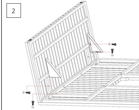
3. Mount the two triangular connector pieces H with 4x J and 4x I on the inside of side panel B and tabletop A. Ensure that the closed sides of connector pieces H face outwards.
