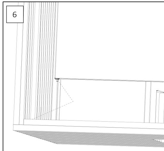
7. The door of the gas cylinder unit **F** can now be installed. Insert the protruding pin of the door into the recess of the frame (tabletop **A**). Hold the door and continue with step 8.
